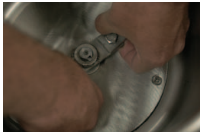
3. Remove worn blade.
