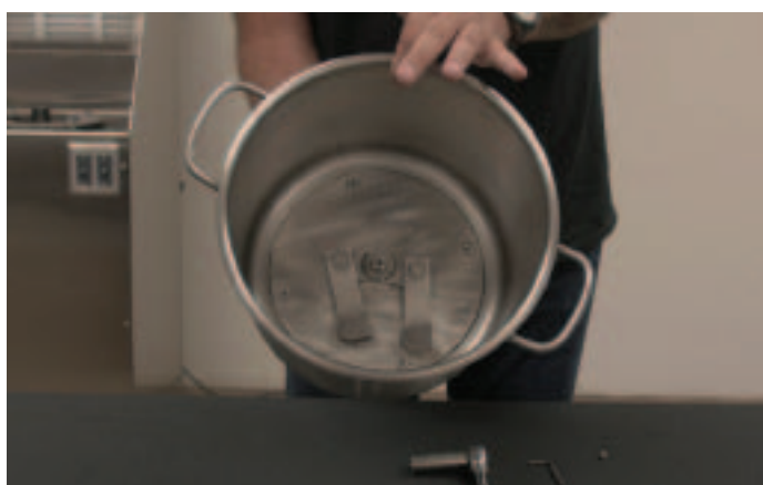
6. Make sure blade lays on top of washer welded to bucket.
