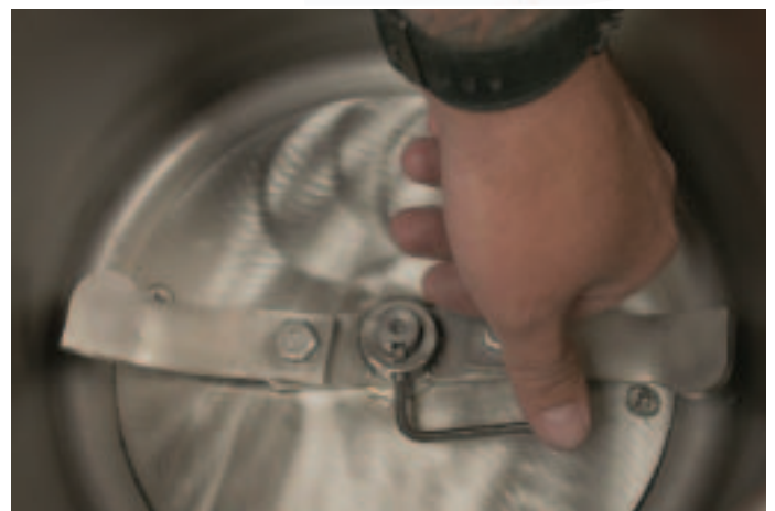
1. Remove set-screw with hex head allen wrench.
