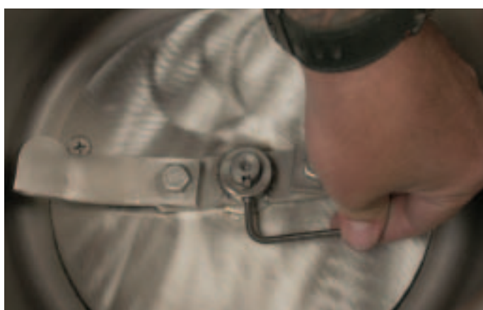
7. Replace set-screw and tighten with allen wrench.
